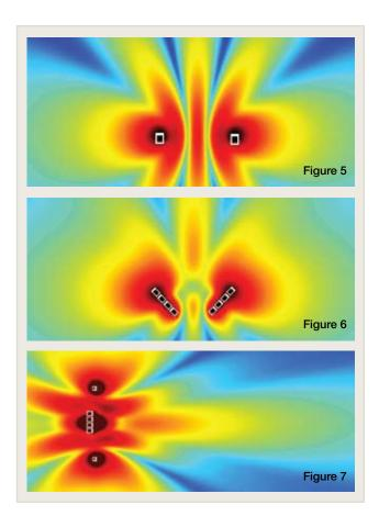
Consider that at the acoustic crossover frequency, by definition the mains and subs are producing equal level. This means that in the crossover region the mains act as a subwoofer system all to themselves! In short, your formerly perfect subwoofer system is now compromised by left- and right-stacked subs anyway, in the form of the main loudspeakers (**Figure 7**).
