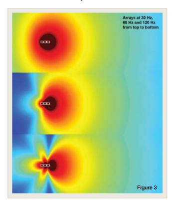
direction of the audience, and then delay each forward subwoofer back to the rearmost. As the energy travels down this line of subwoofers each contributes in time, creating forward addition.
