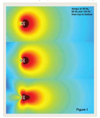
a perfectly functional approximation by taking the cabinet depth and multiplying by two. To convert from distance to delay, remember that sound travels approximately one foot every 0.9 millisecond.
