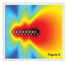
End-fire arrays have their own set of compromises. The primary advantage is near-perfect addition in the forward direction, and the primary disadvantage is the physical space required to implement them.
